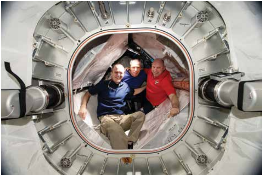
BEAM, the inflatable module attached to the International Space Station, is pioneering the concept of expandable habitats for astronauts. Expedition 55/56 crew members pose for a photo inside the module, which has the advantage of being lightweight yet durable.
